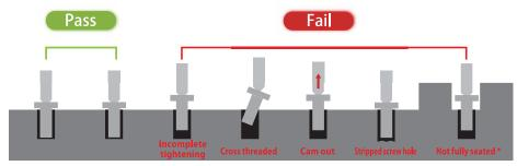
\*If a recess is deep, it is hard to visually notice a not fully seated screw from above
