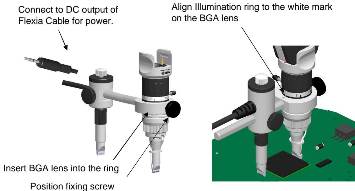
3. Loosen the illumination position screw to move illuminator forward/backward.
