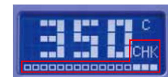
Suction with clogging
