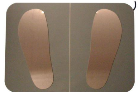
Picture: Footwear electrode for separate shoe testing (350 x 500 x 8 mm)
