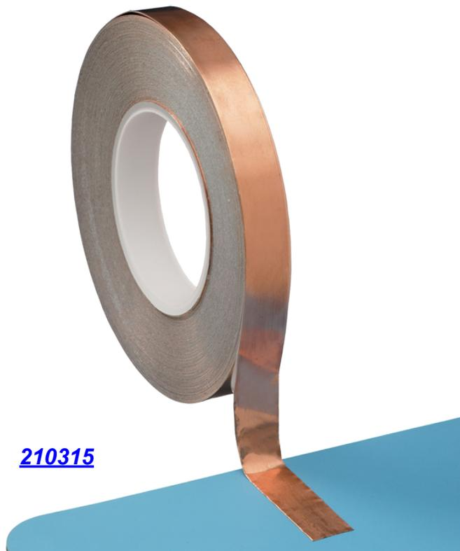
Copper earthing tape is used to ground ESD matting, polishes and paint. The tape is normally laid in strips 4 to 8 metres apart, across the full width of floor, under the floor covering, and then connected to earth protective ground.
