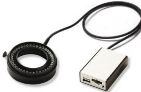
Ring-light containing 40 white LEDs for bright and homogenous illumination of objects. Designed for assembly on Optilia W10x-HD, W20x-HD and M20x-HD cameras. The compact control unit features an ON-OFF switch, brightness control and two outputs for connection to LED illumination units. With Segment control unit, user can toggle 4 groups of LEDs clockwise or anticlockwise.
